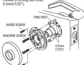
Before assembling the lockset with installing screws, please raise the lever a little and then tighten the screw.
