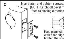
(NOTE: Latchbolt bevel must face to closing direction.)
