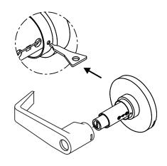
\*For communicating set ensure key is inserted in the north-south position
