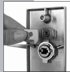
Once the handing is complete, reverse the lever handing stopping block, so that the 'L' shaped locking plate locks down behind the cam assembly, preventing the lever from being rotated back to its original position.
