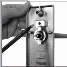
In this instance the trim plate is left handed, this is because the lever is pointing to the side marked 'L'. To change handing, simply undo and remove the screw that holds the lever handing stopping block.
