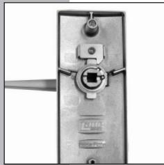
The trim plates supplied are designed to fit back to back on the door. On the under side of each trim plate is printed "**inside plate**" or "**outside plate**". The inside plate is installed to the inside of the door, the side that faces into the home, the outside plate is installed externally.
