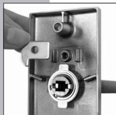
Remove the lever handing stopping block, this will allow the lever to be handed in the opposite direction. You may need to pull down slightly on the lever to assist removing the stopping block.
