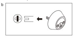
c. Insert two screws through countersunk holes engaging holes in exterior cylinder and tighten firmly.
